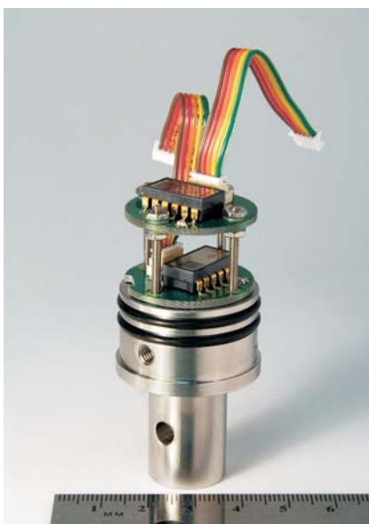
Figure 1. Two MEMS Sensors Mounted 90 Degrees Apart to Create a Geokon Biaxial Tiltmeter.
