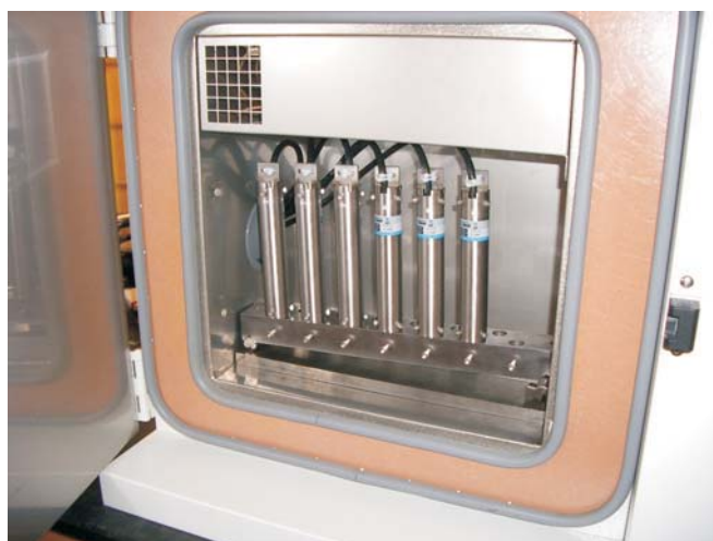
Figure 2. Six tilt sensors and housings on the sine bar for axis A-A inclination in the environmental test chamber.
